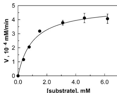
Fig. 3. Plot of the initial hydrolytic rate of BNPP by 1.0 mM  $[\text{Cu}^{2+}\text{-RU}]$  of the 4Vp<sub>3</sub>Ac<sub>1</sub> copolymer at pH 8.0 and 25 °C. The solid curve is the best fit to a pre-equilibrium rate law (Eq. (2)).
