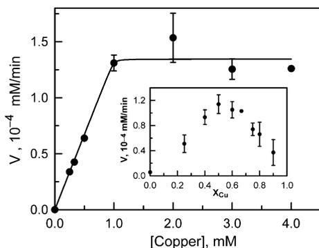
Fig. 2. Titration of  $\text{Cu}^{2+}$  into 1.0 mM RU of 4Vp<sub>3</sub>Ac<sub>1</sub> copolymer, monitored with the activity toward the hydrolysis of 1.0 mM BNPP in 50% methanol solution of 25 mM HEPES at pH 8.0 and 25 °C. Inset shows the “activity Job plot” of  $\text{Cu}^{2+}$ -4Vp<sub>3</sub>Ac<sub>1</sub> in which the initial rate of BNPP hydrolysis (1.0 mM) is plotted against  $X_{\text{Cu}}$  at a constant  $[\text{RU}] + [\text{Cu}^{2+}]$  of 2.0 mM.
