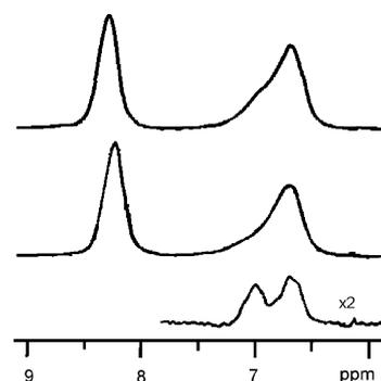
Fig. 1. The  $^1H$  NMR signals of the pyridine ring and the amide  $NH_2$  protons of the copolymer in DMSO (top trace) and in DMSO upon addition of a few drops of  $D_2O$ , where the  $NH_2$  signals are wiped out (middle trace). The change can be clearly seen in the difference spectrum which reveals the  $NH_2$  signals (bottom trace).
