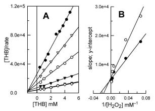
FIG. 6. Hanes analysis of the kinetic data from Fig. 4. The plots in A yield the apparent virtual dissociation constant for THB. The re-plot of the slope and y-intercept from A versus  $1/[H_2O_2]$  reveals (in B) true dissociation constants for THB (0.41 mM) and  $H_2O_2$  (17.3 mM) in a bi-substrate reaction.
