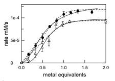
FIG. 8.  $Cu^2$  titration to  $A\beta_{1-20}$  (**A**) and  $A\beta_{1-16}$  (**O**) monitored with their oxidation activities (100 mM HEPES buffer at pH 7.0 and 25.0 °C). The *dotted curves* show the best fittings to a non-cooperative M+L  $\rightleftharpoons$  ML equilibrium. *Solid curves* are the nonlinear fittings to the Hill equation, which yield Hill coefficients of 1.94 and 3.27 for Cu<sup>2+</sup> binding to  $A\beta_{1-16}$  and  $A\beta_{1-20}$ , respectively.
